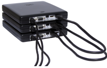
Figure 6.2: 3 Handyscope HS5s combined
