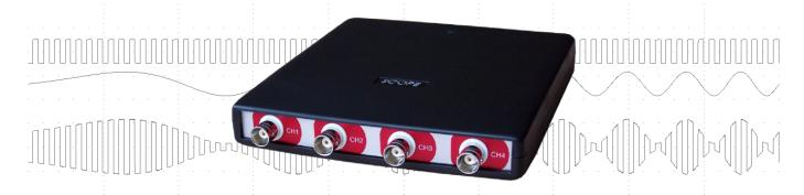
The Handyscope HS4 DIFF is a four channel differential USB oscilloscope with a maximum sampling speed of 50 MSa/s and 128 KSamples memory per channel. The differential input channels enable safely measuring, without risk of creating a short circuit through the oscilloscope. The Handyscope HS4 DIFF is delivered with a complete measurement software package that offers all you need for your measurement applications.
