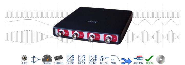
The **Handyscope HS4 DIFF** is a four channel differential USB oscilloscope with a maximum sampling speed of 50 MSa/s and 128 KSamples memory per channel. The differential input channels enable safely measuring, without risk of creating a short circuit through the oscilloscope. The **Handyscope HS4 DIFF** is delivered with a complete measurement software package that offers all you need for your measurement applications.
