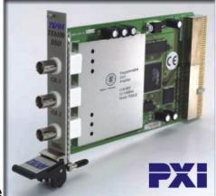
The TE6100 is the first 100 MS/SEC measuring instrument that consists of a Digital Storage Oscilloscope, Spectrum Analyzer, Transient recorder and Voltmeter. This new PXI based, compact measuring instrument, can solve almost every measurement problem. Analyzing signals is done with an 8-bit resolution and a maximum sampling speed of 100 MHz. The input ranges 0.1 volt full scale to 80 Volt full scale. The record length is 32K/64K samples.
