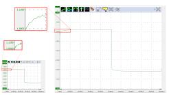
Shown are two displays, both showing a measurement of the same signal. The left display size corresponds to a size comparable to a standalone oscilloscope; at 8 bit resolution, zooming will not reveal more details. The right display corresponds to a maximized window on a standard PC screen; at 14 bit resolution, zooming will still reveal more details.
