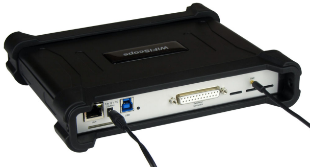
Figure 7.2: Rear ground connection
