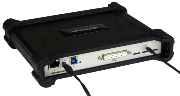
Figure 7.2: Rear ground connection
