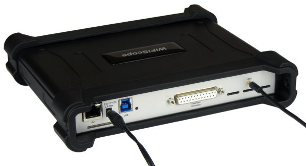
Figure 7.2: Rear ground connection
