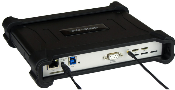
Figure 7.2: Rear ground connection
