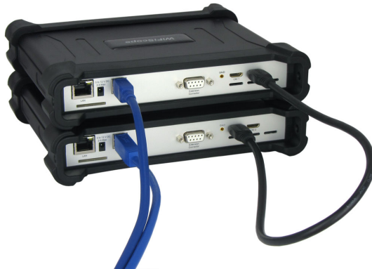
Figure 8.3: Multiple ATS WiFiScopes combined
