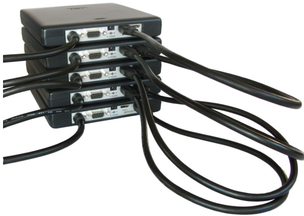
Figure 6.3: Multiple Automotive Test Scope ATS6s combined
