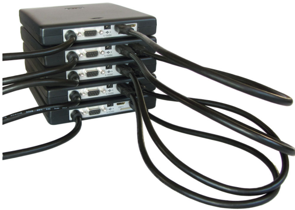
Figure 6.3: Multiple Handyscope HS6s combined
