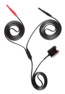
The Measure lead TP-C812C is a low noise differential measure lead designed to be used with the Handyscope TP450. This 2 meter long measure lead splits in two individual ends of each 1.2 meter long. The dual banana socket connector at one end plugs directly on the european mains plug adapter that can be attached to the instrument. The two other ends each feature a single 4 mm banana plug, on which application specific test points, clamps or probes can be plugged.
