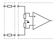
The Differential attenuator TP-DA10 can simply be placed directly on the input of the instrument and the measuring lead on the other end of the attenuator.
