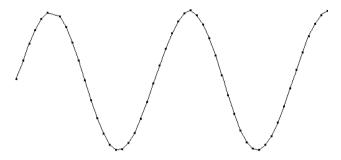
The more samples are taken, the better the signal can be reconstructed. The sampling frequency must be higher than 2 times the highest frequency in the input signal. This is called the Nyquist frequency. Theoretically it is possible to reconstruct the input signal with more than 2 samples. In practice, 10 to 20 samples are necessary to be able to examine the signal thoroughly.
