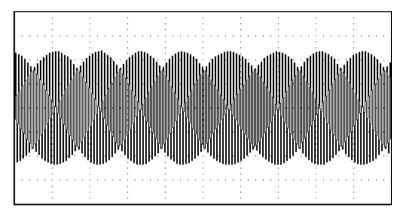
This time it is a sine wave signal with a frequency of 257 kHz, which is sampled at a frequency of 50 kHz. The minimal sampling frequency should have been 514 kHz. For proper analysis, the sampling frequency should have been 5 Mhz.
