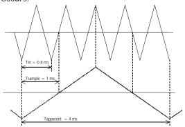
The input signal is a triangular signal with a frequency of 1.25 kHz (upper most in the illustration). The signal is sampled at a frquency of 1 kHz. The dotted signal is the result of the reconstruction. From that triangular signal the periodical time is 4 ms, which corresponds with an apparent frequency (alias) of 250 Hz (1.25 kHz - 1 kHz).
