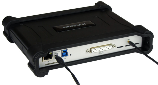
Figure 7.2: Rear ground connection
