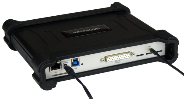
Figure 7.2: Rear ground connection
