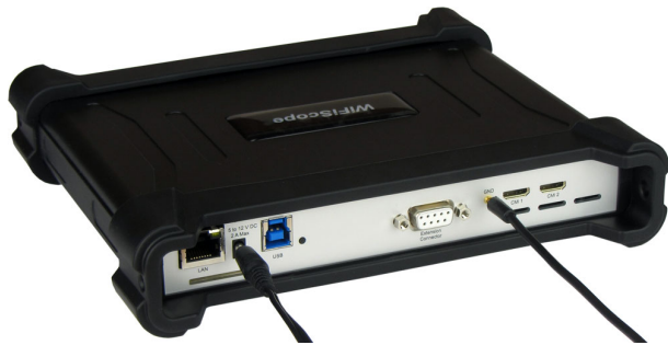
Figure 7.2: Rear ground connection
