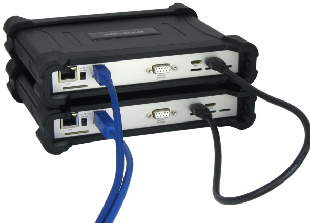
Figure 7.3: Multiple WiFiScope WS6s combined
