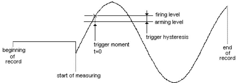
The input signal is compared with two levels in the trigger system: the arming level and the firing level. When the input signal passes the arming level, the trigger system is armed. If the input signal passes the firing level, the trigger system becomes active and 'fires' a pulse. This pulse is used to start the display of the signal.
