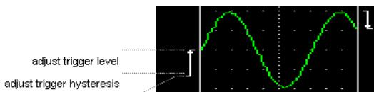
In the above picture, the trigger mode of the left hand symbol is set to Rising slope and the trigger mode of the right hand symbol is set to Falling slope.
