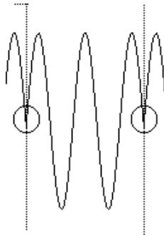
This means that because of the calculation errors extra frequency components are generated around the true frequency. Because of this 'smearing' the amplitude of the true frequency decreases, since the area under the curve remains the same.
