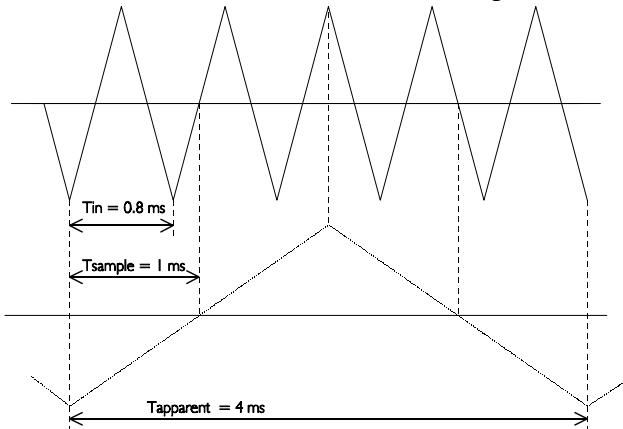
The input signal is a triangular signal with a frequency of 1.25 kHz (upper most in the illustration). The signal is sampled at a frequency of 1 kHz. The dotted signal is the result of the reconstruction. From that triangular signal the periodical time is 4 ms, which corresponds with an apparent frequency (alias) of 250 Hz (1.25 kHz - 1 kHz).
