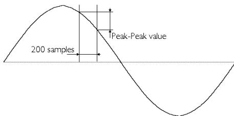
If the time in which the 200 samples are taken is too long in relation to the periodical time of the input signal, **aliasing** can occur (see also the chapter about the oscilloscope).
