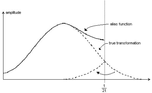
The original signal is sampled at a sample time  $t$ . The critical frequency (Nyquist frequency) is  $(1/2t)$  Hz.
