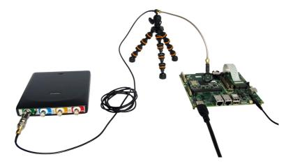
In the Multi Channel software, select an EMI Quick Setup to setup the instrument and software properly for performing the EMI pre compliance test measurements.
